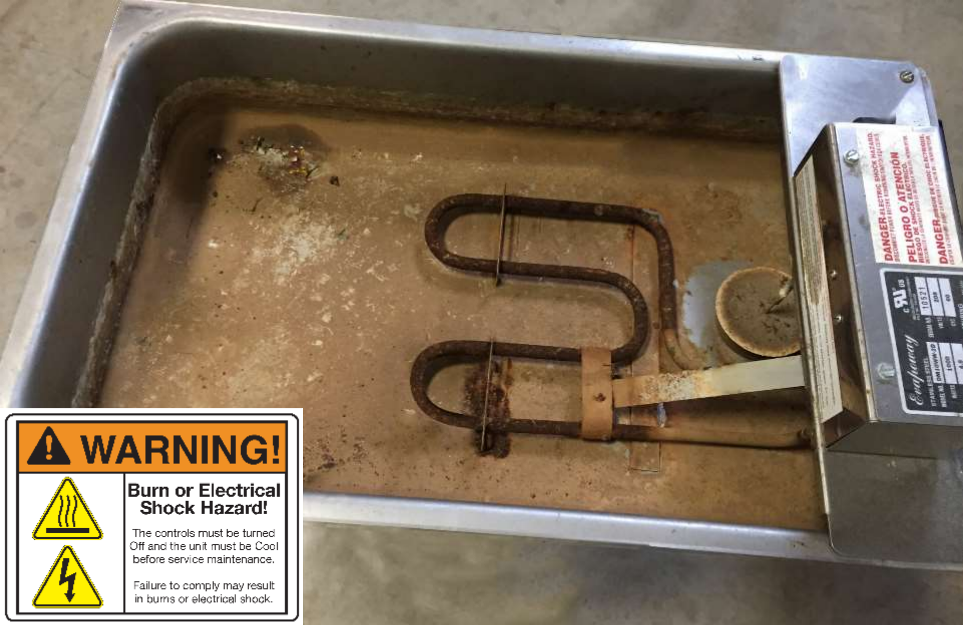
Inspect and clean the evapoway pan if needed. Shut down the power and allow the water to cool before cleaning.
